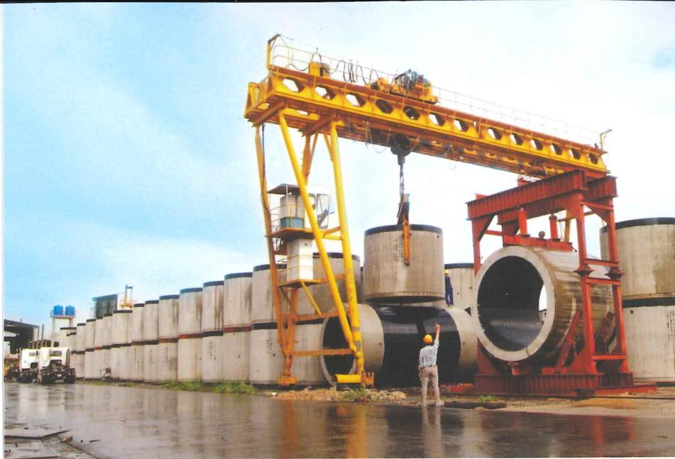
Concrete grade made for pipe jacking is very high, minimum grade is 55 MPa. Depending the condition of waste water, jacking pipe will be manufactured which include/exclude PVC liner or using suitable cement and admixture for mixing concrete. At Hung Vuong company, jacking pipe with diameter from 500mm to 3000mm are produced by core vibration technology (Jumbo machine from Germany) and hitting vibration technology (Italian technology).
